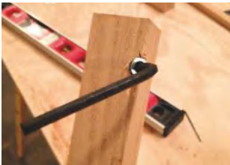
STEP 6. The legs are then attached using a bolt
